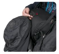
A buckle on the cockpit holds up the cocoon during take-off.
